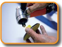
In order to replace the back pad, we had to use a wrench. To save time and trouble, we used the same backing pad to polish the flat and curved surfaces. When polishing the flat surface with the original backing bad, the wave pattern remains on the surface. And, the original backing pad was a little bit hard for polishing the curved surface and could not take advantages of flexible diamonds. Therefore, we created the new backing pad for flat surfaces.
