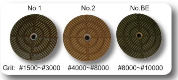
Size: 5, 6, 8, 10 inch Grid: No.1, No.2, No.BE By adopting the original resin bond, this pad made it possible to polish a point with excellent cutting force and long life. Polish the stone with the regular pad up to the step #800, and then use Super Flat for the last 3 steps. It can save time and meantime, you can obtain the natural shine.
