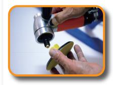
In order to replace the back pad, we had to use a wrench. To save time and trouble, we used the same backing pad to polish the flat and curved surfaces. When polishing the flat surface with the original backing bad, the wave pattern remains on the surface. And, the original backing pad was a little bit hard for polishing the curved surface and could not take advantages of flexible diamonds. Therefore, we created the new backing pad for flat surfaces.
